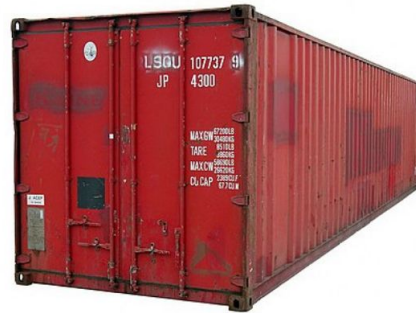
A 40-foot long (12.19 m) shipping container. Each of the eight corners has an essential twistlock fitting for hoisting, stacking, and securing
